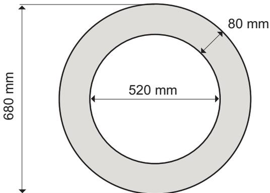
Minimum hole for the flange is 570 mm
