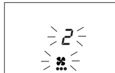
The selected level can be seen by the points under the fan icon on the screen.
