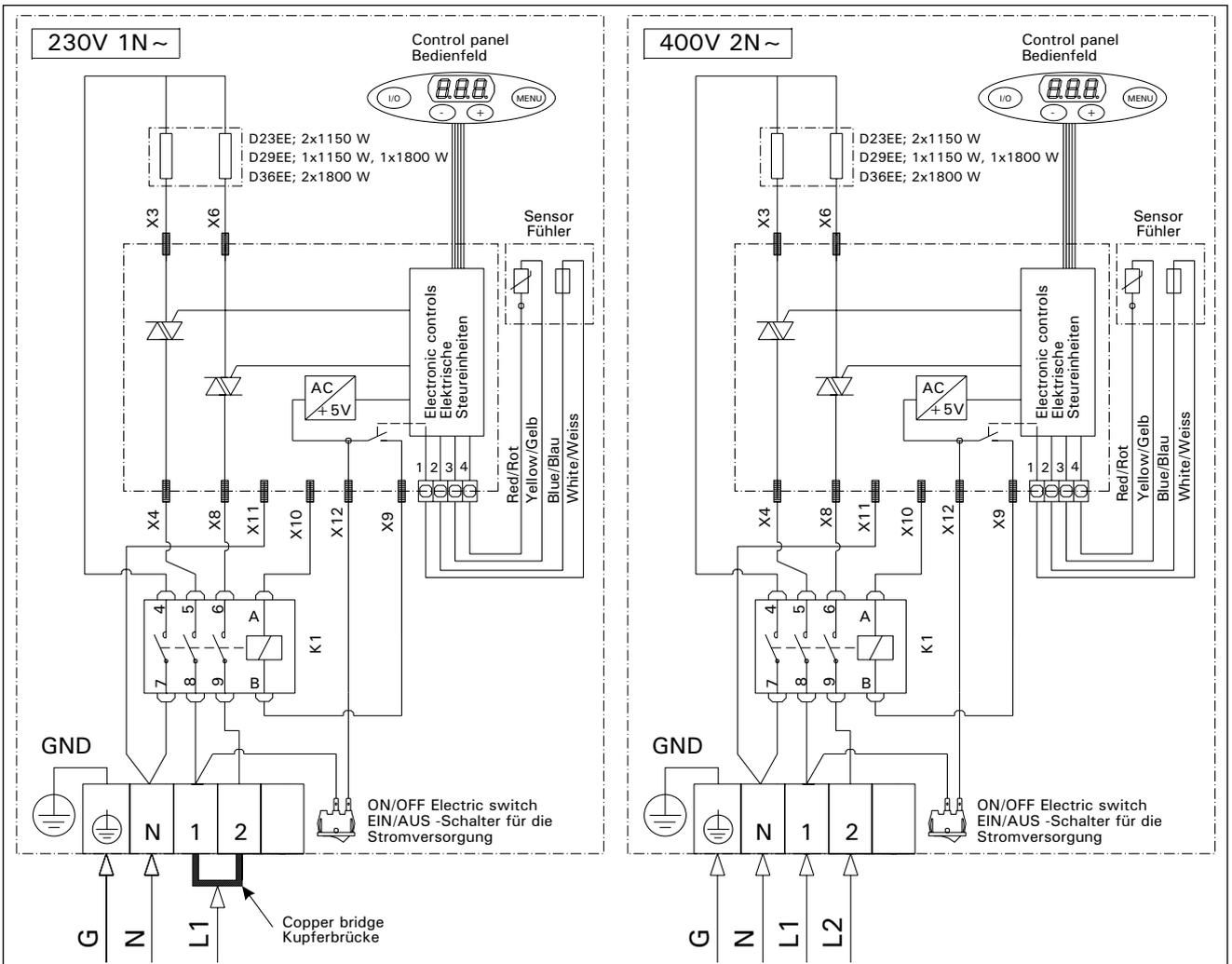
Figure 9a. 1-phase connection of the heater
