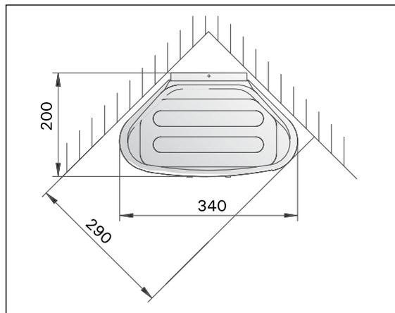
**Figure 4. Dimensions of heater**
