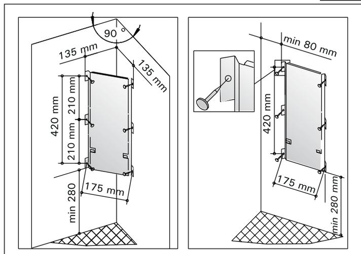
**Figure 6. Location of the mounting rack of the heater**
