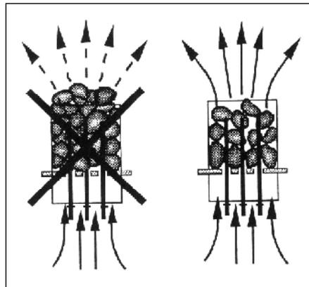
Figure 1. Piling of the sauna stones
