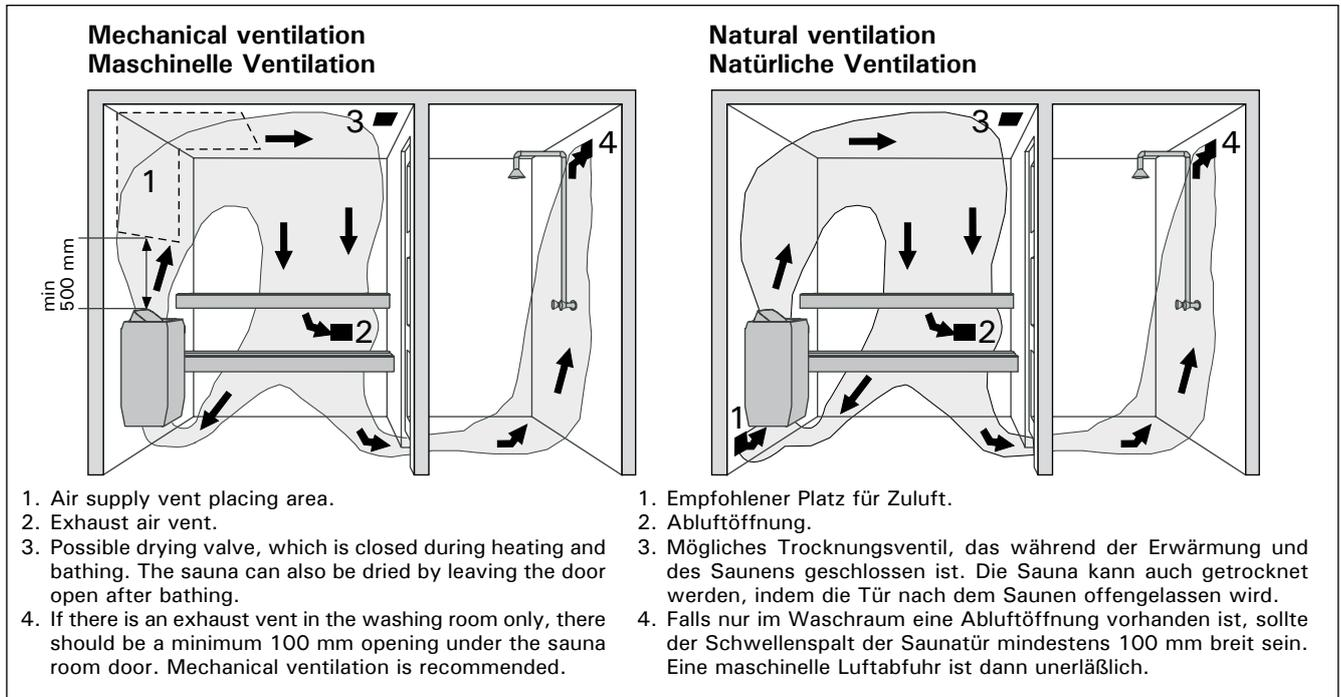
**Figure 3. Ventilation of the sauna room**
