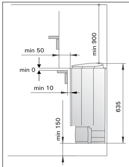
**Figure 5. Safety distances from the heater**
