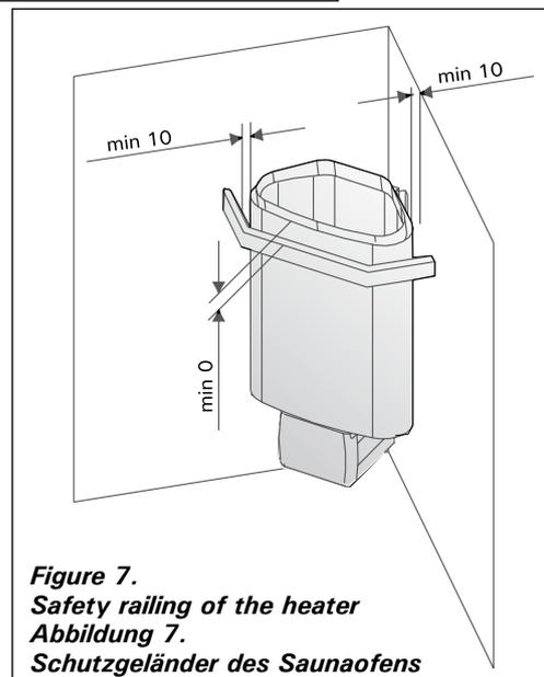
**Figure 7. Safety railing of the heater**
