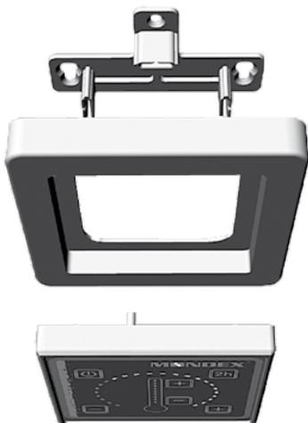
The wall mounting plate is either mounted with three screws to the wall or fixed to the bottom of the mounting box. The mounting plate is covered with a cover plate and finally with the control panel. The mounting cable is 8 m. Cut the extra cable and connect the other end to the heater. When installing the control panel, make sure that the cables are not detached or deformed.
