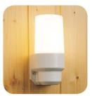
Sauna lamp 40 W (Art. 9001 1000) Wall-mounted. White lamp-holder E14. IP 24. Max 40 W. Ø 90 mm, Height 170 mm.
