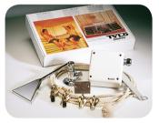
Water sprinkler (Art. 9034 1000) An innovative solution for sprinkling water over hot sauna stones. Connect to hot or cold water. Consists of a 7-metre twined hemp rope running through brass eyebolts, a sprinkler head, a valve box with lever and a rope bolt, together with plumbing connections. Supplied in a gift package with an exclusive bronze plaque.
