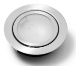
**Downlight** (Art. no. 9001 1081) Effective spotlighting for recessed installation in, for example, a soffit outside the sauna. (Not suitable for use inside the sauna.) 12 V/5 W. Connect to our 12 V transformer. Installation size: dia. 60 mm. IP 21
