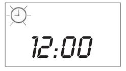
You may now set the current time using the  $\checkmark$  and  $\blacktriangle$  buttons during the blinking of the clock symbol.
