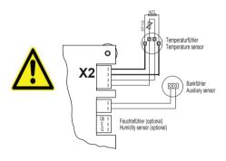
If the sensor is connected correctly, the control unit shall automatically recognise it once the mains voltage has been switched on again. By faults of the second sensor the following error messages will be displayed:
