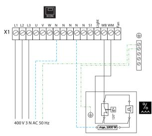
Caution: When connecting the vaporizer the output "W" is switched from the sauna heater to the terminal "Wb" to the vaporizer. In this case, the sauna
