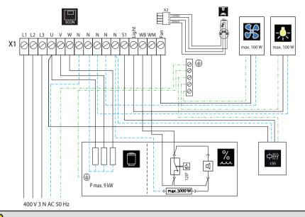
Warning: Always connect the neutral terminal (N) of the sauna oven. During steam operation, one phase of the oven is switched off; therefore the power load will no longer be symmetrical. The result is that the neutral wire is no longer current-free.
