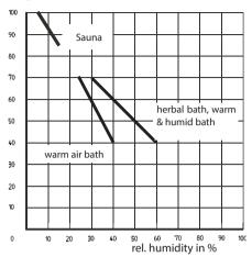
Without connection of the optional humidity sensor the humidity intensity shown in the display corresponds to the time proportional vaporizer setting. Therefore, the relative air humidity is not preselected or shown on the display in such case, but rather the switch-on frequency of the vaporizer in percent. The below diagram is intended to clarify this.
