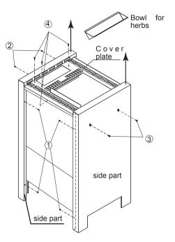
Now slide the 7 individual soapstone plates, as illustrated, from above with the grooves on the fixing rail.
