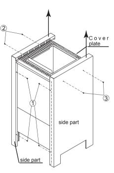
Now slide the 7 individual soapstone plates, as illustrated, from above with the grooves on the fixing rail.
