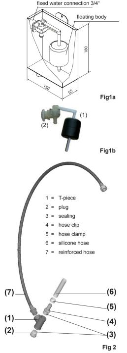
Put before mounted adapter-piece with the hose-nozzle into the open end of the silicone-hose. Secure it with the hoseclamp.
