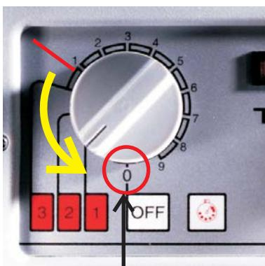
... Then back again to the figure corresponding to length of time you wish the heater to run for (3, 2 or 1 hours).
