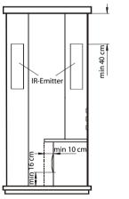
For assembly, a right-angled opening must be fitted vertically into the wood.
