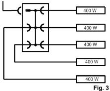
An additional clamping distribution with order no. 94 2046 must be used for fitting 6-9 infrared emitters.
