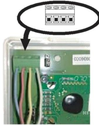
The control unit is connected with the sauna heater by means of a 4-pin silicone cable. The wall sensor is connected with the same type of cables. Both cables are delivered in one piece, so that the sensor has already been mounted to one end. The cable has to be cut through in the suitable place, so that it would be of suitable length. The total length of the cable in the set is 14 m.
