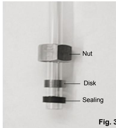
Insert glass tube into screw connections. Screw nut on crimp connection with moderate stress.
