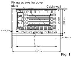
1. Screw 4 fixing screws acc. Fig. 2 into the cabin wall over the air inlet opening so that there is still 3 mm clearance between the wall and the screw head.
