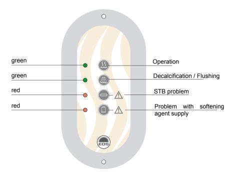
The LED "operation" lights up when the sauna equipment is in operation, independently of whether the steam generator is working or not.
