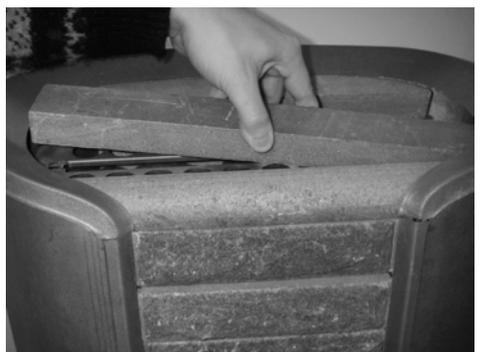
Finally check that the soapstones are between the end limiters and that the gaps between the stones are equal.
