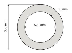
Minimum hole for the flange is 570 mm
