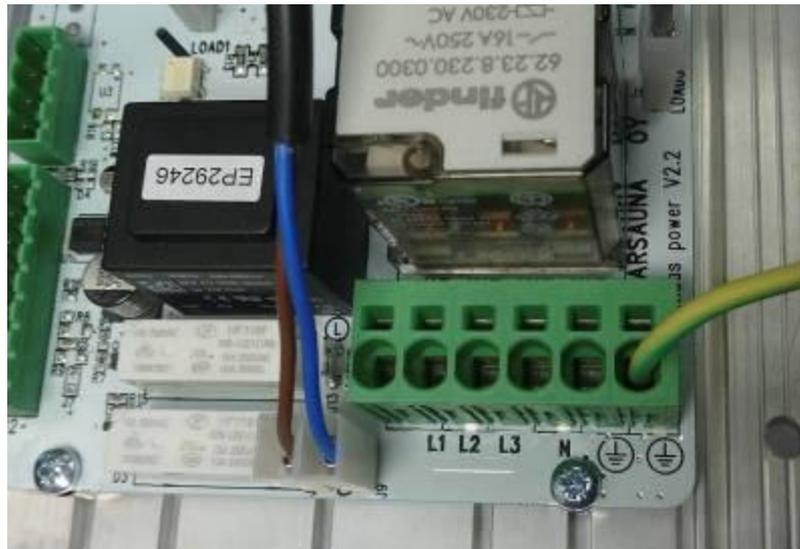
5. **Temperature reduction (Connector J5)** (If this feature is in use, it is possible to connect a relay or contactor coil to the output, which control the heating of the building) Detach the connector from the circuit card and screw the cables to the connector. Then, press the connector back onto the circuit card. The screws will point right when pressing the connector.
