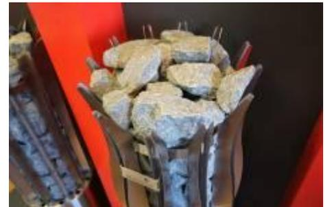
6. Pile the upper part with stones until you have reached approx. 5 – 10 cm from the top of the resistors. Lower the upper resistor plate in its place, and finish piling stones in the sauna stove. Ensure that there are enough stones on top. It is recommended to choose big stones for the top of the sauna stove, so that they cannot fall through the vertical profiles.
