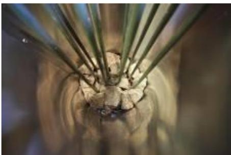
2. Pile the stones into the lower part of the sauna stoves. Do not wedge the resistors. Ensure that the resistors travel vertically where they have been attached to the bottom plate, throughout the entire section where the stones have been installed. Stop piling stones when you reach the end of the middle part of the resistor, and move to Section 3.
