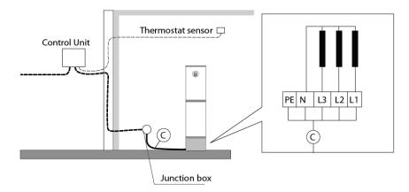
Heater's electrical connection, double input
