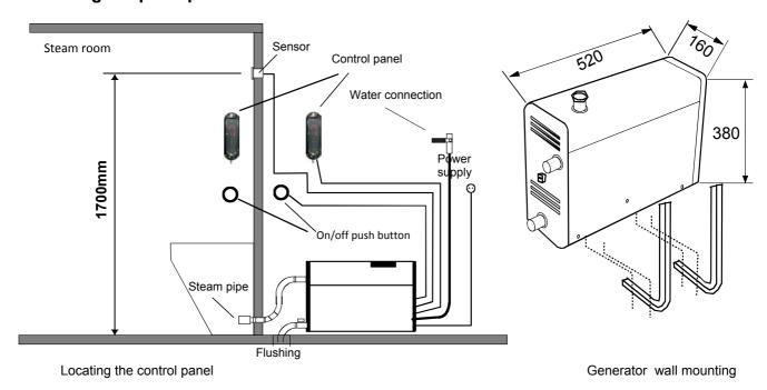
Control panel is installed inside or outside the steam room, model HNS – M2.
