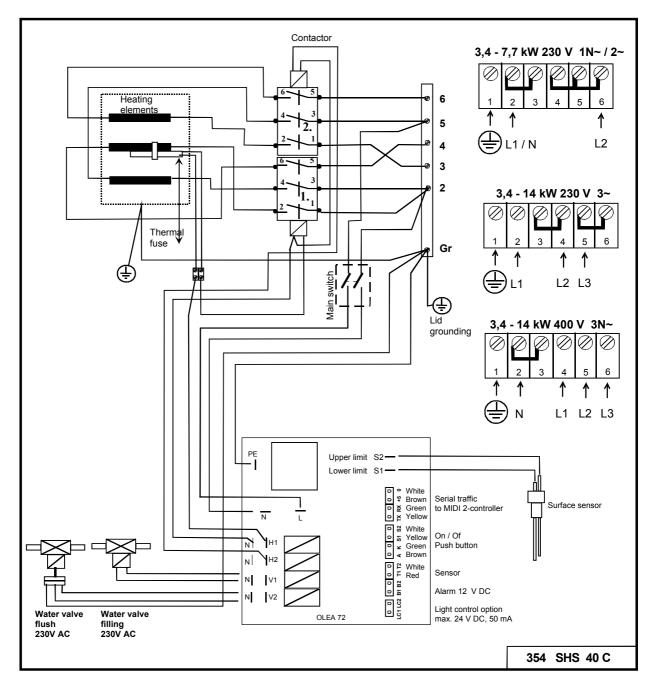
HNS – M2 3,4-7,7 kW  $230V - 240V 1N^{\sim} / 2^{\sim},$   $230V 3^{\sim},$   $400V - 415V 3N^{\sim}$  HNS – M2 9,5-14,0 kW  $230V 3^{\sim},$   $400V - 415V 3N^{\sim}$
