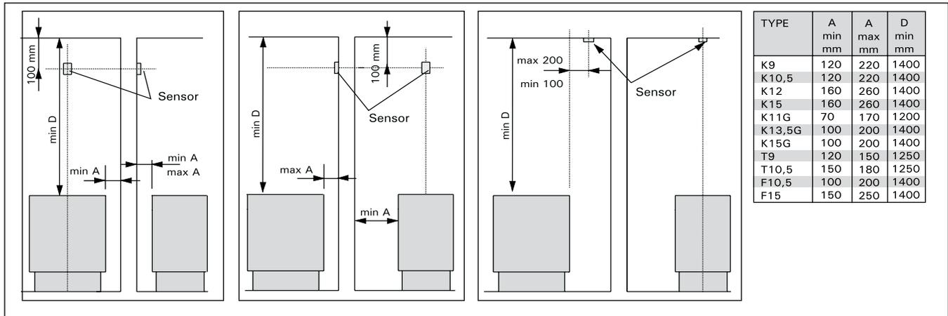
**Figure 31.** The position of the sensor box of the control unit C150VKK in connection with heaters attached to the floor.
