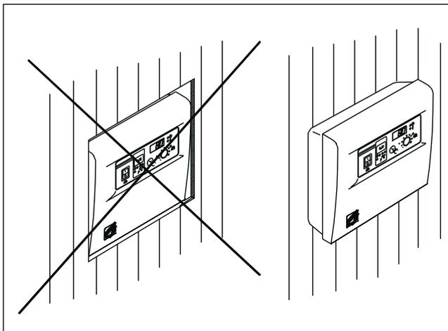
Figure 24. Wall-mounting the control unit
