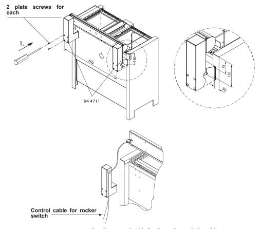
Lay the control cable for the rocker switch and heater supply with a minimum clearance of 30 mm.
