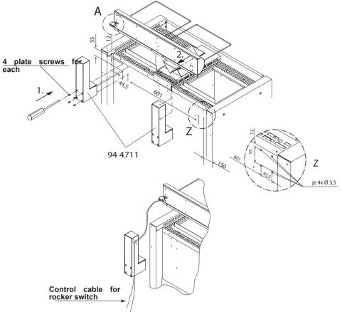
Lay the control cable for the rocker switch and heater supply with a minimum clearance of 30 mm.
