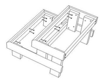
8) Secure the front edge of the rear using the screws as shown in the figure.
