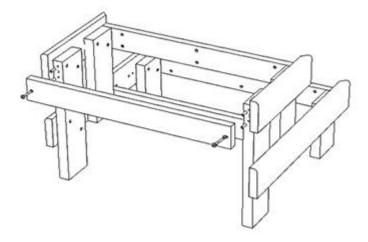
3) Attach the fixing part without slot to the back side of the second step (Do not forget the dowels).
