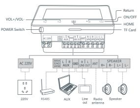
3.1.Guidance of system installation wiring constructionThe installation of this system requires integrated wiring. All the connecting lines must be pre-buried into the wall with universal electrician pipes.Therefore, the system integrated wiring work must be synchronized with the room.waterand electricity decoration wiring work.
