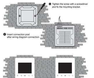
After connecting the cable,put it into the bottom box, align it with the position of the bracket, press it in, and then finish the installation after hearing the jam. Disassemble the machine
