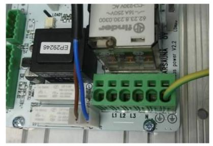
5. **Temperature reduction (Connector J5)** (If this feature is in use, it is possible to connect a relay or contactor coil to the output, which control the heating of the building) Detach the connector from the circuit card and screw the cables to the connector. Then, press the connector back onto the circuit card. The screws will point right when pressing the connector.
