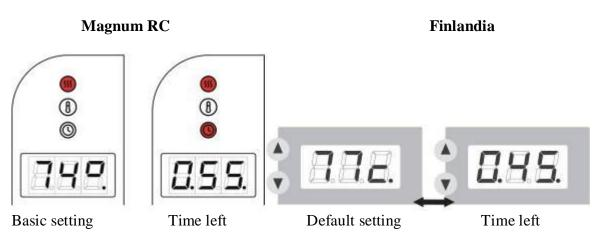
When the machine is on, the default mode and the remaining time alternate on the screen with an interval of approximately 10 seconds.
