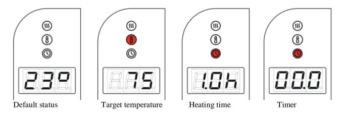
The adjustment menus of the device are shown in the above image. The user can move from one menu to another using the Menu button. When the sauna stove is on, the (+) and (-) buttons may be used to move to the mode where you can adjust the settings in the order shown in the image above.
