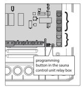
By SteamRock Premium generator the programming button is on the main board next to the sauna bus connector.
