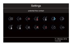
Tap two times on the symbol to open PFC settings. A submenu with the choice of synchronisation options shown like symbols will open. By choosing one of these symbols you can assign the PFC a certain synchronisation scenario relative to some other functions of the control unit, e.g. main heating or light switching in order to operate the external equipment in the desired way.
