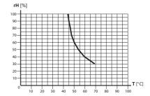
and under the curve may be selected. For instance at 60°C temperature your can set up to 40% rel. air humidity. In order to set a higher humidity you will need first to reduce the temperature.
