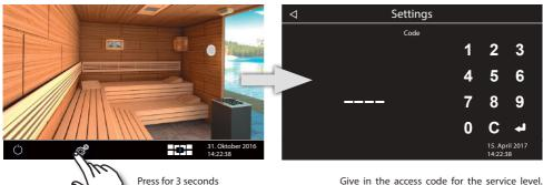
Give in the access code for the service level. Correction with "C". Confirm entry with the "enter" button.
