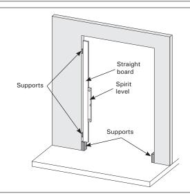
4. Fasten the top part of the frame to the side parts. Lift the frame into the opening in the wall. Leave a gap of about 10 mm between the top of the frame and the opening. It is recommended to leave 100–200 mm gap under the door for ventilation in the sauna (about 10 mm in other rooms).
