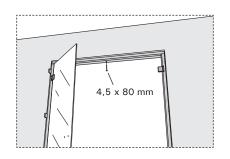
**9.** Cut off the excess parts of the wedges if necessary (saw in a vertical position). Remove the supports.
