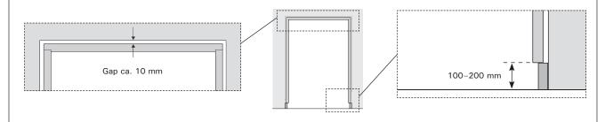
Tip! You can make the installation easier by installing temporary stoppers to the supports so that the door can lean on them. This is especially recommended if you are working alone. To be able to install the cornice strips correctly, place the stoppers so that the flagging on the wall and the door frame are on the same level.
