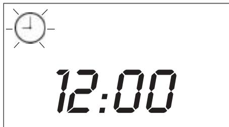
You may now set the current time using the ▼ and ▲ buttons during the blinking of the clock symbol.
