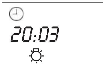
When the pre-selected start-up time is reached, the sauna switches itself on. After the designated heating time it then shuts itself back off automatically.
