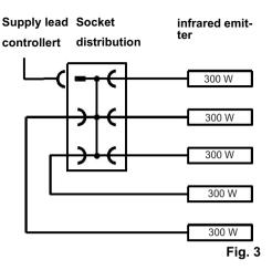
An additional clamping distribution with order no. 94 2046 must be used for fitting 6-9 infrared emitters.
