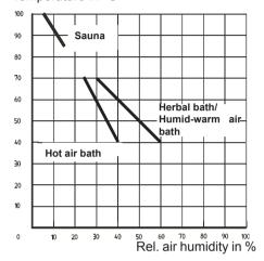
The humidity intensity shown in the display corresponds to the time proportional evaporator setting. Therefore, the relative air humidity is <u>not</u> preselected or shown on the display, but rather the switch-on frequency of the evaporator in percent. The graphic is intended to clarify this.
