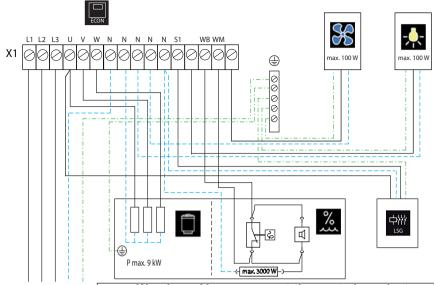
Warning: Always connect the neutral conductor of the sauna oven. During steam operation, one phase of the oven is shut down; therefore the heating load is no longer symmetrical. The result is that the neutral wire is no longer current-free.
