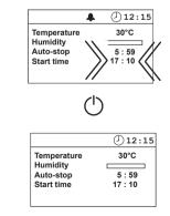
If the sauna unit is to be used without preselection time, --: -- must be entered in the display under preselection time.
