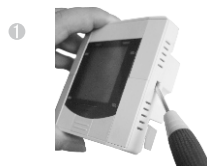
Twist the screws at the bottom
