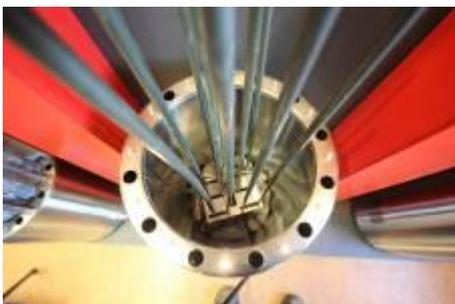
3. Lower the resistor plate onto the stones as shown on the images, and continue piling the stones. It is very important to pile stones properly between the resistors, and for the resistors to be aligned straight. This ensures that the resistors cannot bend against each other, which might otherwise cause the resistors to break. However, do not put too many stones
