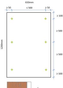
Measure and accurately mark the locations of the mounting points to be drilled in the slabs. Observe the minimum edge distances: ≥ 50 mm on the vertical side and ≥ 100 mm on the horizontal side. When installed on the ceiling, the maximum distance between the fasteners is 400 mm.
