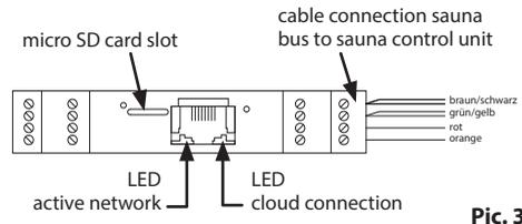
The module housing has a cap rail mounting and if necessary may be mounted on the appropriate rail either next to the sauna control unit (recommended) or next to the internet access point (e.g. router).
