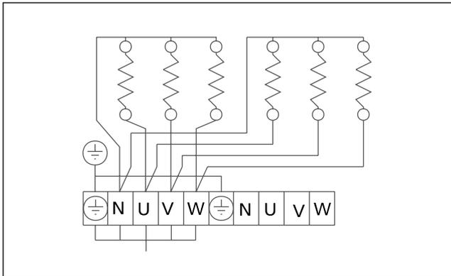
Figure 5. The heater's electrical connections
