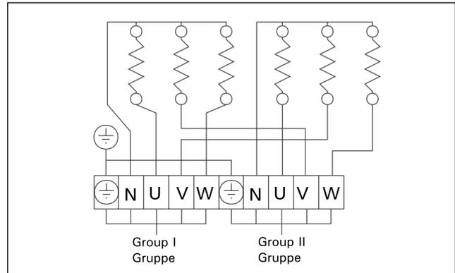
Figure 6. The heater's electrical connections in two groups
