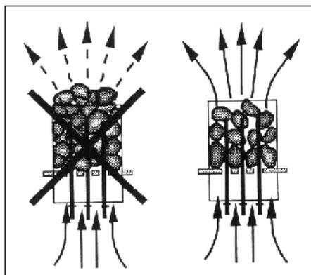
Figure 1. Piling of the sauna stones
