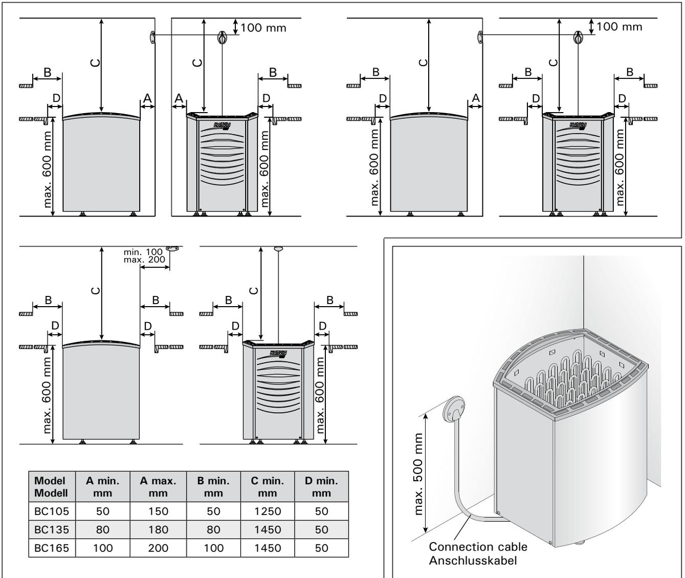
Figure 3. The heater's safety distances
