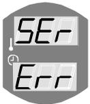
SEr Err (Serial Error) serial traffic error between the heater and the controller.
