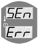
SEn Err (Sensor Error) stone space element disconnected or damaged.
