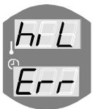
hiL Err (High Limit Error) stone space overheated (>400°C), electronic disconnection.
