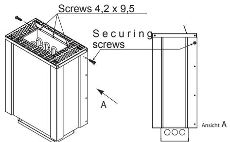
4. Install the terminal block back into the original position in the heater and fasten it with two screws.
