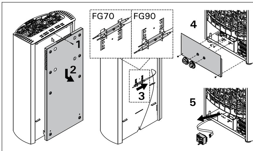
Figure 11. Replacing the thermostat
