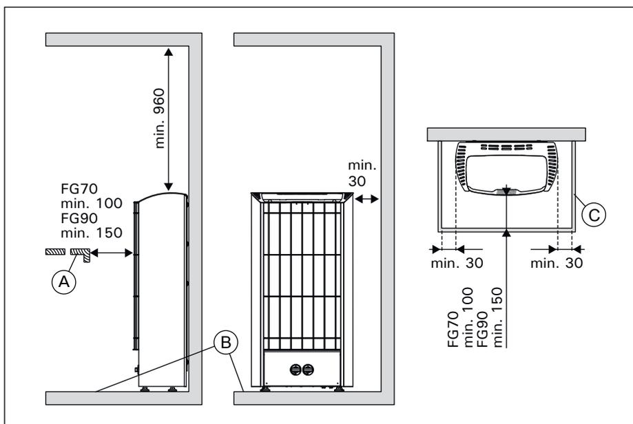
**Figure 6. Safety distances (all dimensions in millimeters)**
