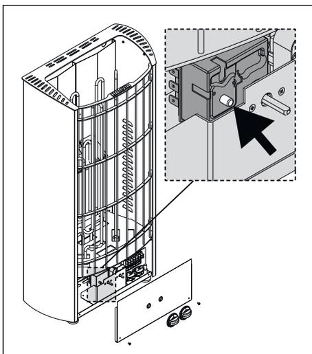
Figure 10. Reset button for overheat protector
