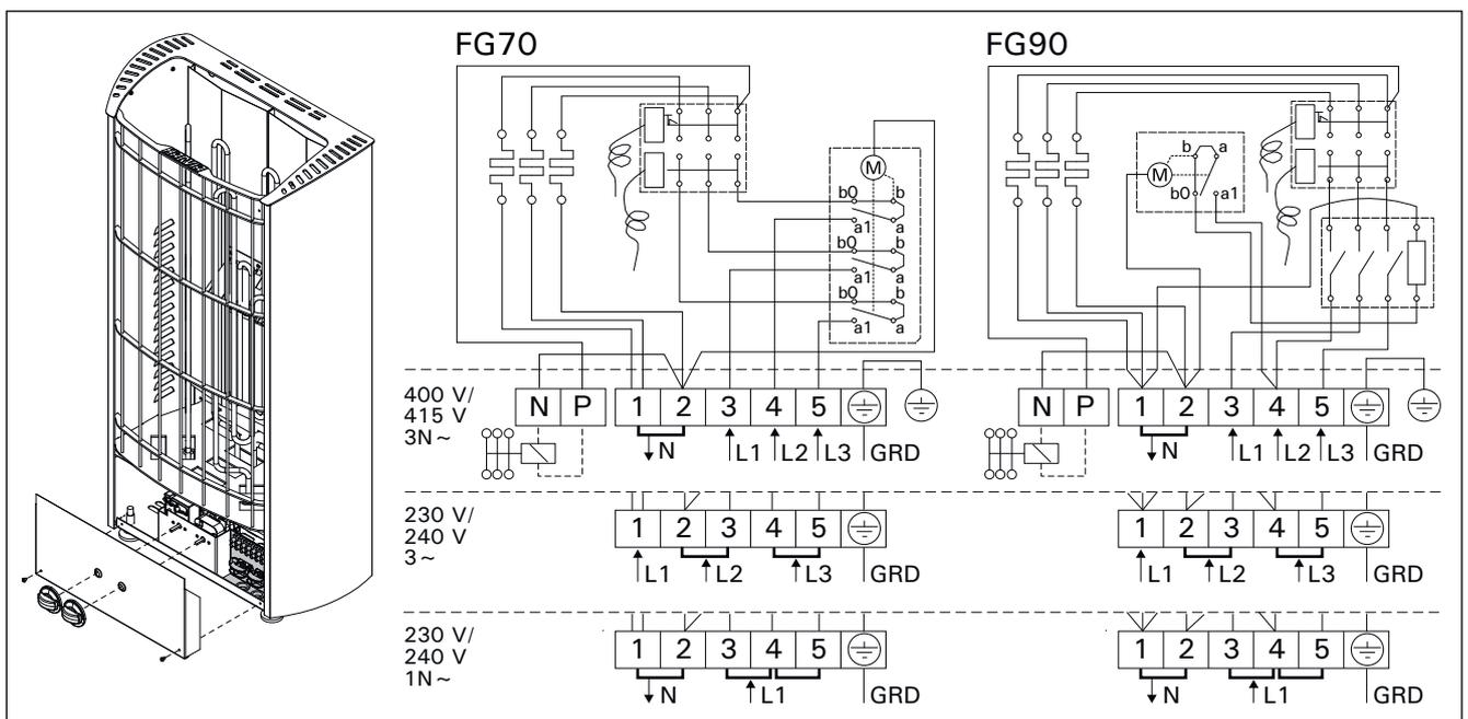
Figure 9. Electrical connections
