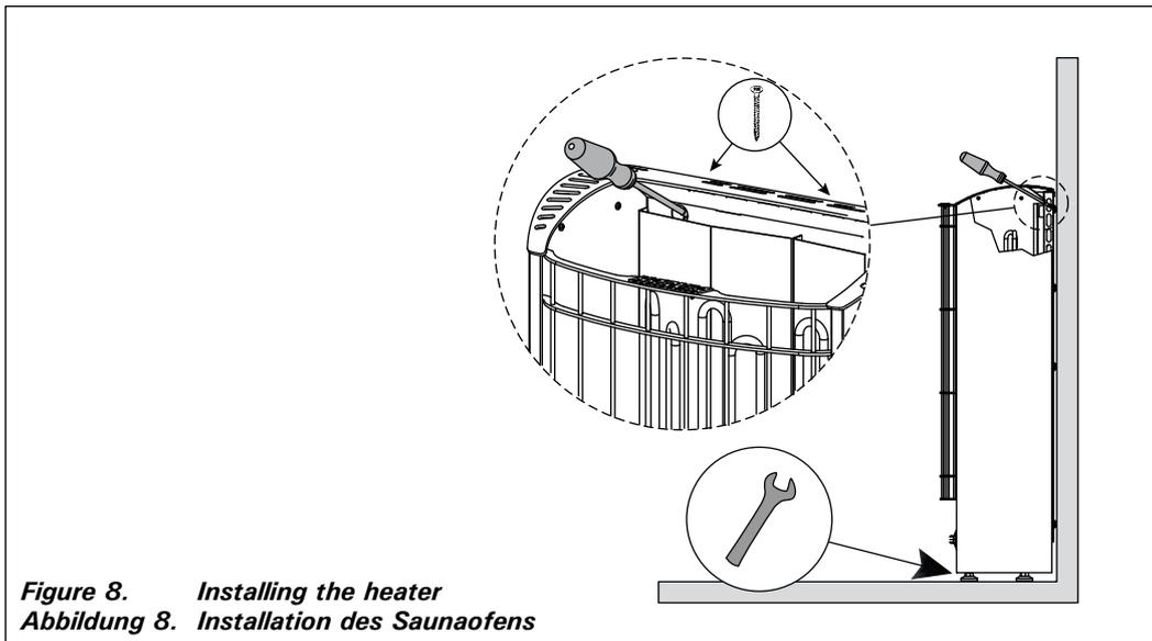
Figure 8. Installing the heater
